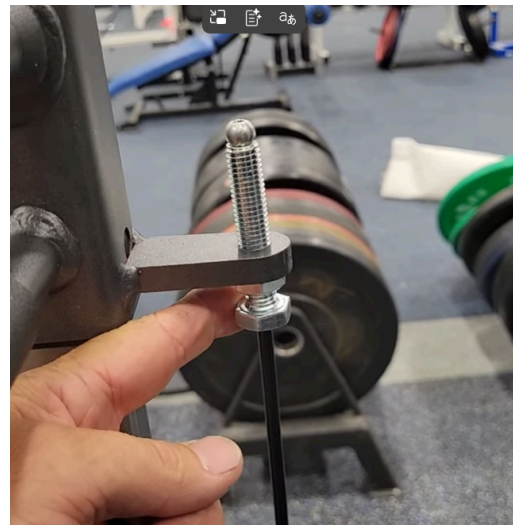
End of cable attachment coming up from the bottom
